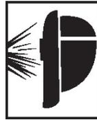
This symbol indicates that the helmet must be worn during the step(s) that follow to protect against eye damage and burns due to flash hazard.
