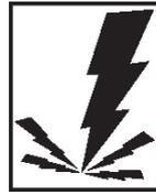
This symbol indicates that the possibility of electric shock hazard exists during the operation of the step(s) that follow.
