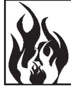
This symbol indicates that the possibility of fire hazard exists during the operation of the step(s) that follow.
