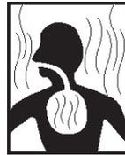
This symbol indicates that the possibility of toxic gas hazard exists during operation of the step(s) that follow.
