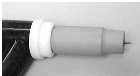
Fig 9 – Tungsten Stickout
