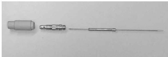
Fig 8 – Assembly order for Torch Parts
